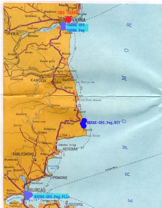
Fig. 3: Connection of EUVN GPS stations, tide gauges and levelling benchmarks
